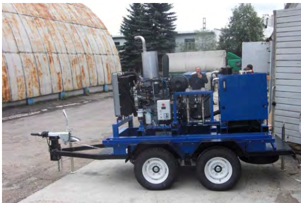
Hydraulic station for GNS-362DR, with additional option on wheel-trailed base
